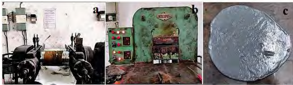
Fig 1. (a) Mixing Mill; (b) Mould Press; (c) Rubber mixed Compound
